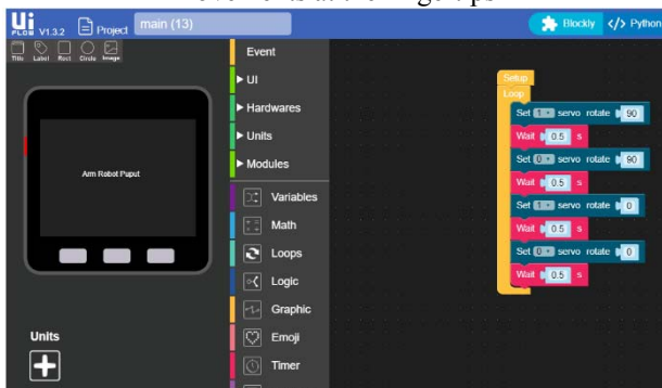
Fig.14 initialize the timer to adjust the speed of the robot finger movement
