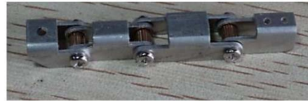
Fig 4. robot finger forming components
