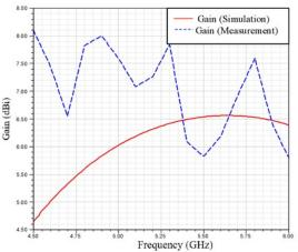
Fig. 7. The gain value comparison of the measurement and the simulation microstrip antenna
