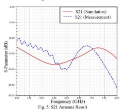
S11 and S21 have good agreement return loss values to obtain from the simulation and measurement the value of S11 and S21 simulation is -19.84 dB and 18.51 dB. The value of S11 and S21 measurement is -21.47 dB and -17.39 dB. This antenna has a gain value 5.82 dBi. To draw the graphics properties of far-field antenna radiation from as a function of spatial coordinates (three dimensions) [14]. It is necessary to know the antenna radiation pattern. Following Figure is the antenna radiation pattern:
