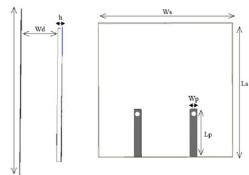
Fig. 1. Structure of the microstrip antenna (a) Front, (b) Side, (c) Rear
