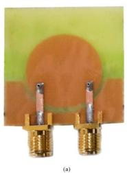
Fig. 3. Physical structure of the microstrip antenna
