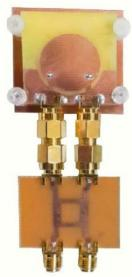
Fig. 11. 900 phase difference 5.5 Ghz microstrip antenna integration
