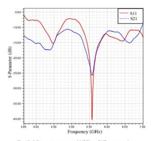
Fig. 12. S-Parameter antenna and 90° Phase Difference coupler integeration
