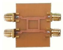
Fig. 8. Implemented 90° Phase Difference coupler
