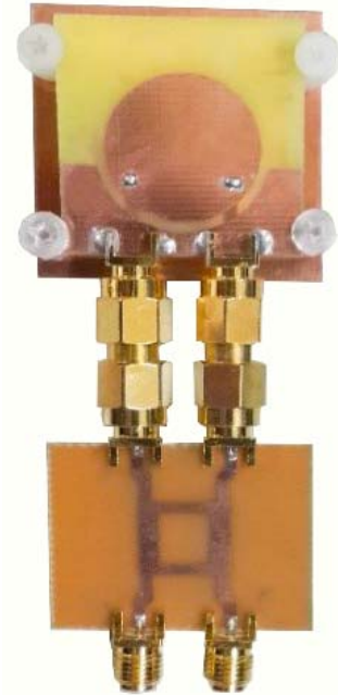
Fig. 11. 90° phase difference 5.5 GHz microstrip antenna integration
