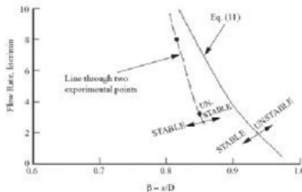
Gambar 9. Perubahan *Flow Rate* Terhadap *Pinch Ratio* (Pejack, 2006)
