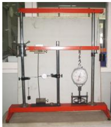
Gambar 4. Alat Uji Buckling
