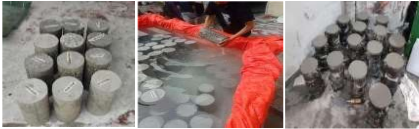
Gambar LII.4. Proses Perawatan Beton Non Pasir
