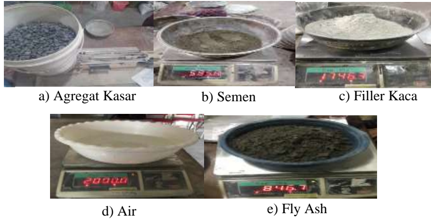
Gambar LII.1 Penimbangan Material Beton Non Pasir
