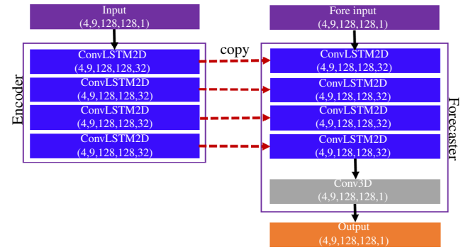
Fig. 6. Configuration of DConvLSTM model
