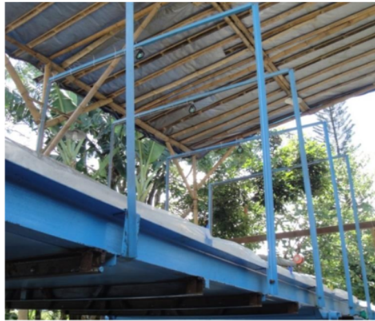
Figure 2. Rainfall simulator with 5 sprinklers and 1 m-distance sprinkler frame.
