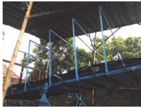
Photo 1. The tilted plot and the 5-sprinklers rainfall simulator (phot. L. Sedyowati)
