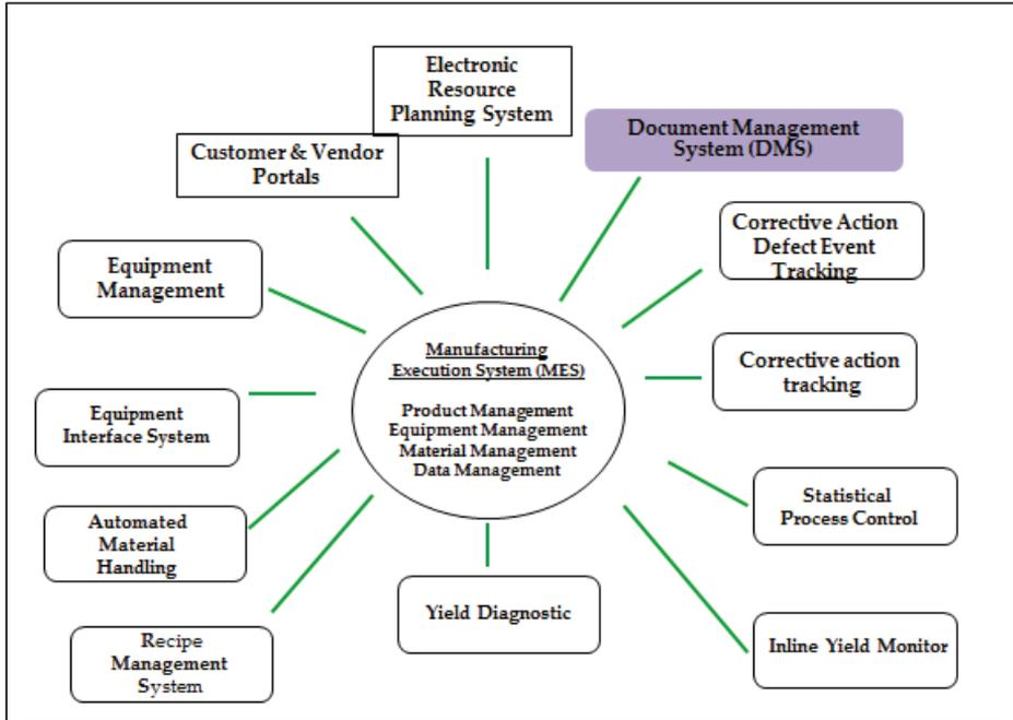
Figure 1: Interlinked manufacturing execution system
