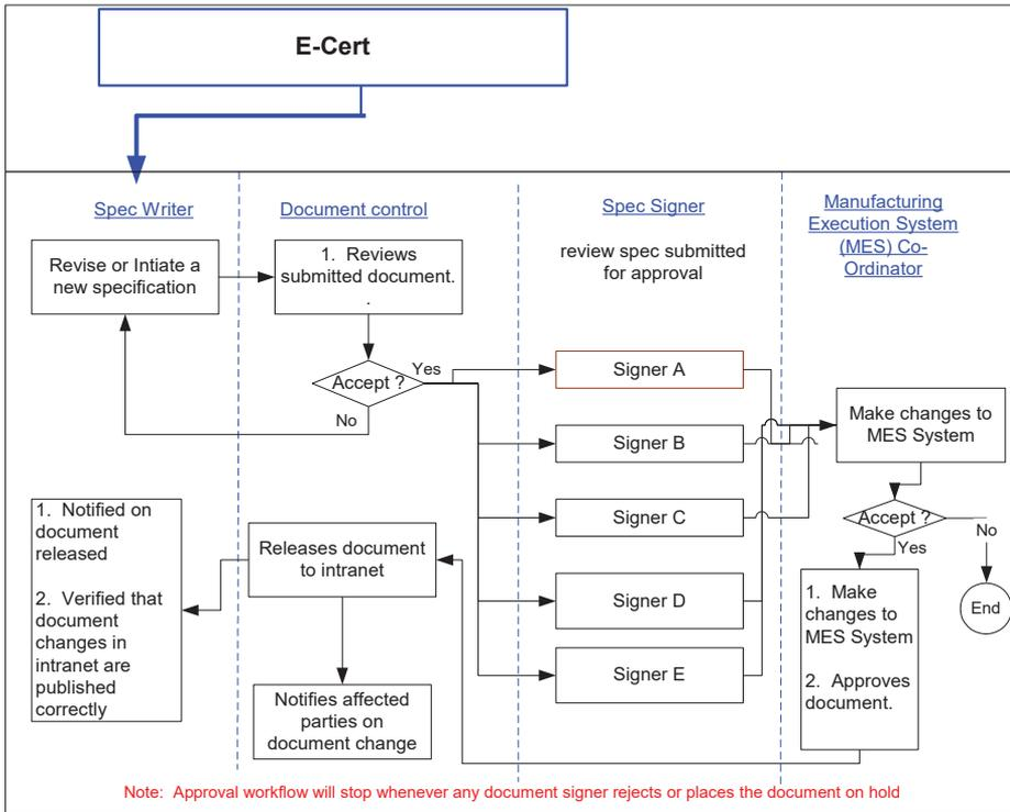
Figure 4: Proposed framework for new workflow approval
