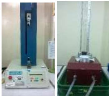
Figure 6: Tensile Strength and Translucent Strength Test Equipment
