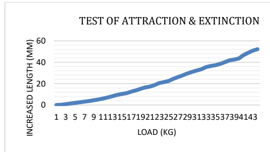
Figure 14: Load Test Graph of PVC Tarpaulin Fabric
