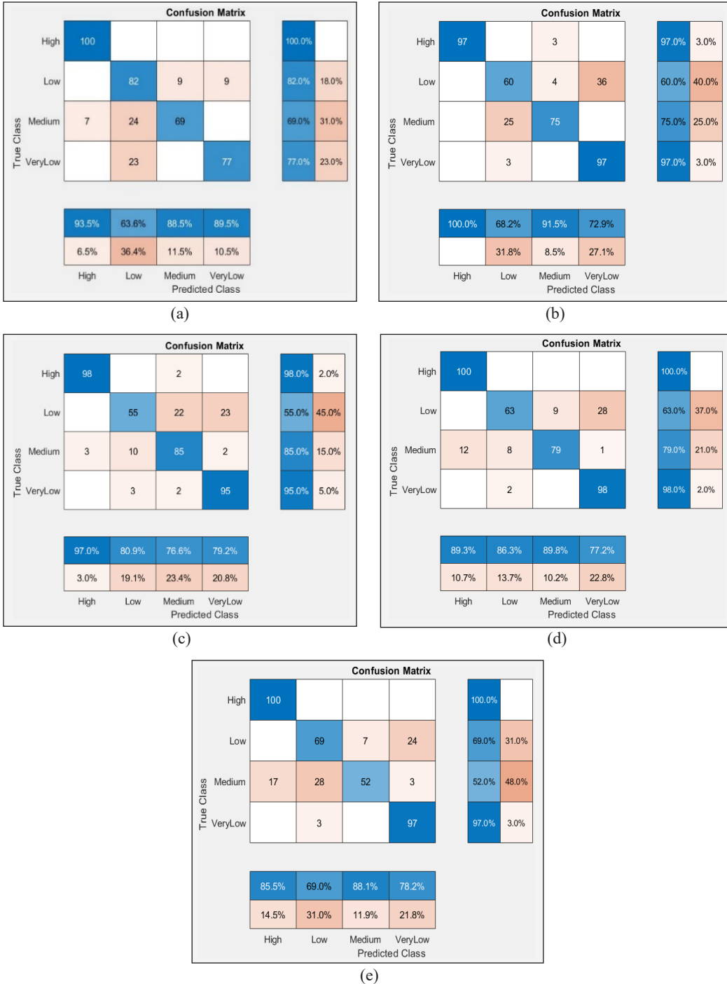
Figure 5. Confusion matrix of testing data: (a) GoogLeNet (optimizer = Adam, learning rate = 0.00005); (b) GoogLeNet (optimizer = Adam, learning rate = 0.0001); (c) GoogLeNet (optimizer = RMSProp, learning rate = 0.0001); (d) ResNet-50 (optimizer = RMSProp, learning rate = 0.0001); (e) ResNet-50 (optimizer = Adam, learning rate = 0.0001)
