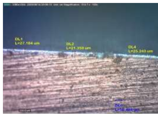
Figure 5. The oxide coating thickness resulted from the anodizing process with a 100% solution type 1M Sulfuric acid ( H_3PO_4 ) with a voltage variation of 15 Volt and immersion time of 30 minutes using an optical microscope 100x
