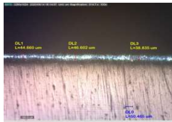
Figure 3. The oxide coating thickness resulted from the anodizing process with a 100% solution type 1M Sulfuric acid ( H_2SO_4 ) with a voltage variation of 30 Volt and immersion time of 10 minutes using an optical microscope 100x
