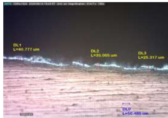
Figure 7. The oxide coating thickness resulted from the anodizing process with a 100% solution type 1M Sulfuric acid ( HNO_3 ) with a voltage variation of 15 Volt and immersion time of 10 minutes using a 100x optical microscope
