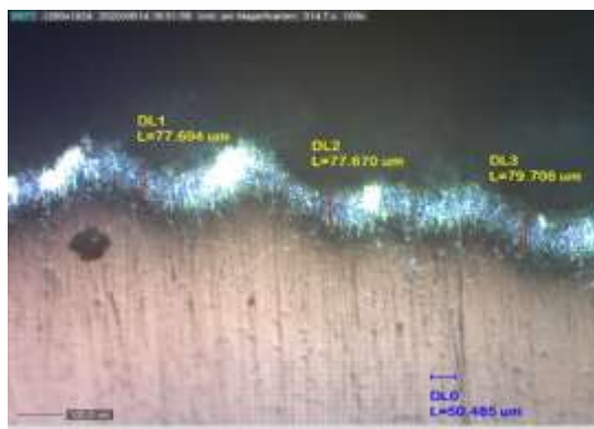
Figure 8. The oxide coating thickness resulted from the anodizing process with a 100% solution type 1M Sulfuric acid ( \text{HNO}_3 ) with a voltage variation of 15 Volt and immersion time of 30 minutes using a 100x optical microscope
