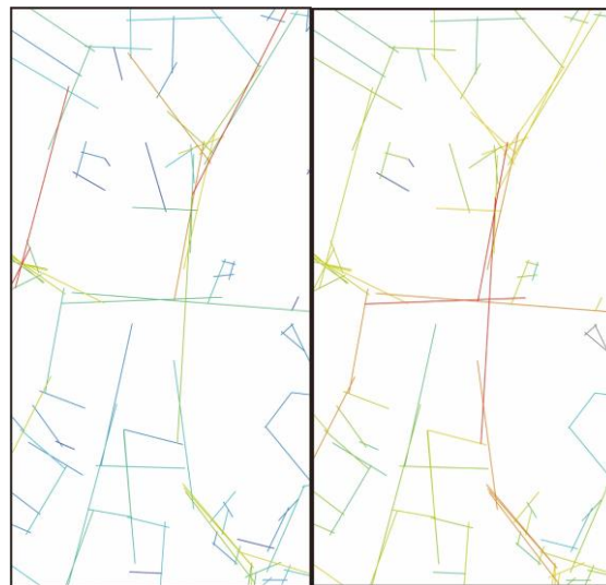
Figure 4. Connectivity line (Left) and Integration (HH) line (Right) (Source: DepthMap Calculation)
