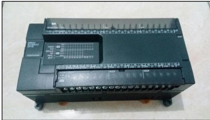
**Gambar 2.1.** PLC Omron CP1E E60 SDR-A
