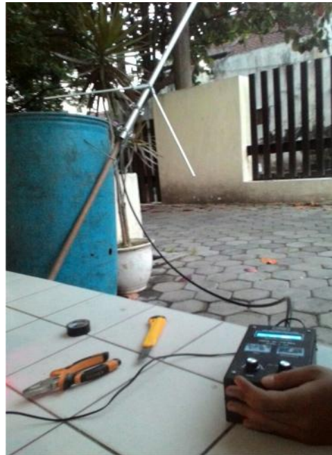
Figure 2.12 Connect the Antenna with SWR meter
