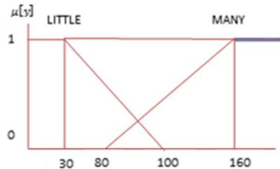
Fig. 3. Membership function “Capacity” Boss Limited
