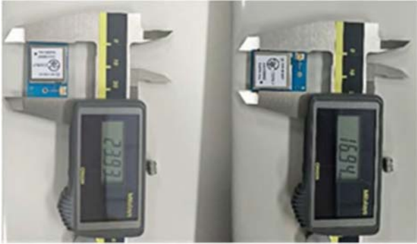
Fig. 2. ES920LR Dimension (MeRL Data)
