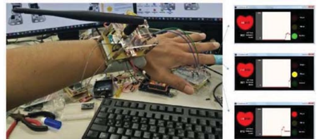
Fig. 7. Prototype ES920LR LoRa
