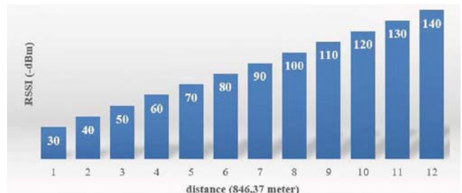
Fig. 11. RSSI on Hill obstacles 846.37-meter Tx-Rx
