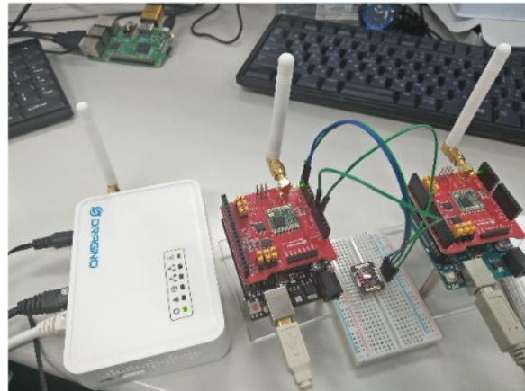
Fig. 15. LoRa Gateway, LoRa Tx and LoRa Rx.
