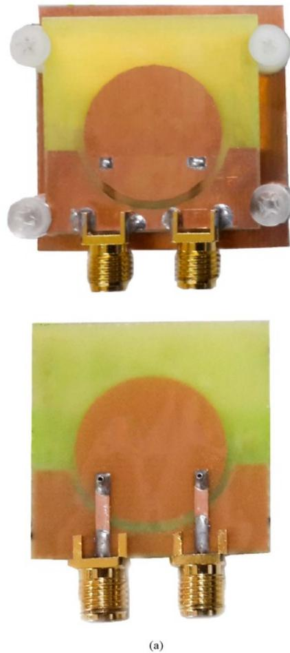
Fig. 3. Physical structure of the microstrip antenna
