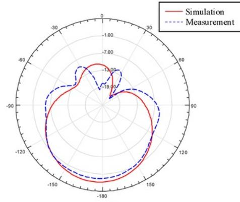
Fig. 6. (a) Theta angles of The radiation pattern, and (b) Phi angles of The radiation pattern
