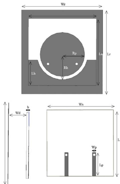
Fig. 1. Structure of the microstrip antenna
