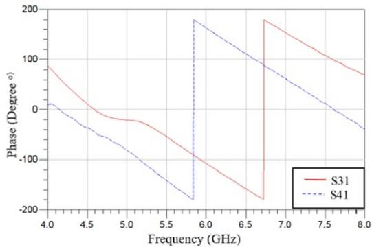
Figure 10. Phase output r 90° phase difference coupler
