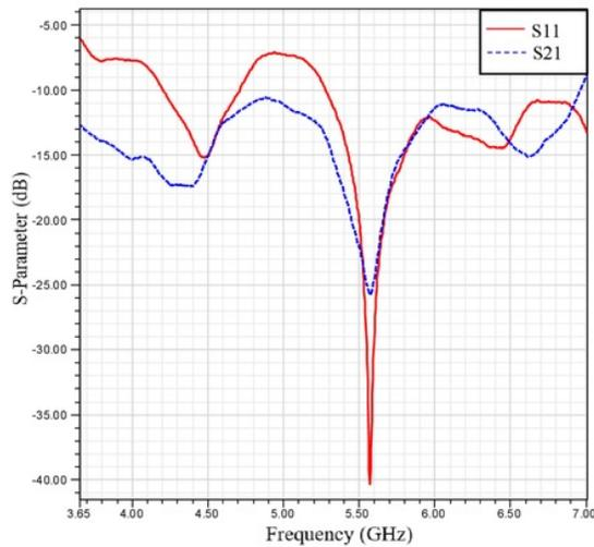
Fig. 12. S-Parameter antenna and 90° Phase Difference coupler intergeration
