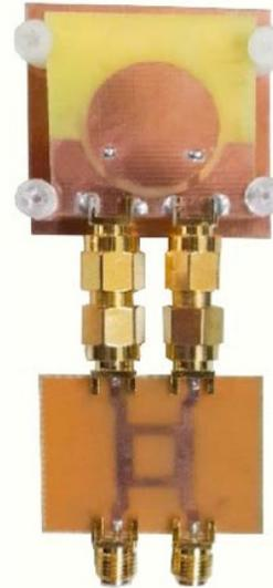
Fig. 11. 90° phase difference 5.5 Ghz microstrip antenna integration
