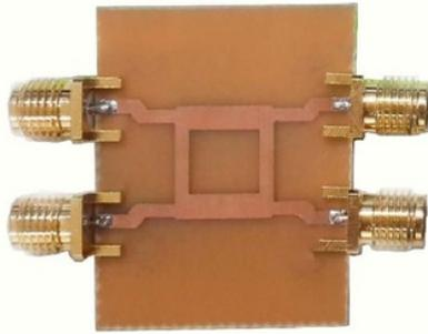
Fig. 8. Implemented 90° Phase Difference coupler
