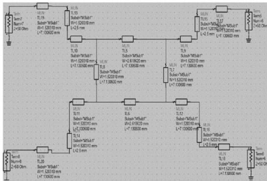
Figure 2. 90° Phase Difference coupler circuit Design
