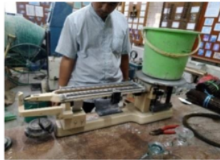
Gambar 4.10 Takar/timbangan Material Campuran Beton
