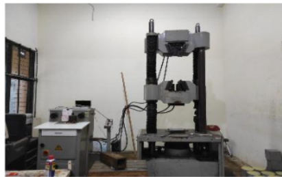
Gambar 4. 20 Alat Uji Kuat Tekan Aksial UTM (Universal Testing Machine)( ASTM C192)
