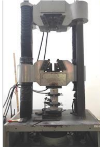
Gambar 4.23 Alat Pengujian Kuat Tekan Aksial Beton UTM ( Universal Testing Machine )( ASTM C192)
