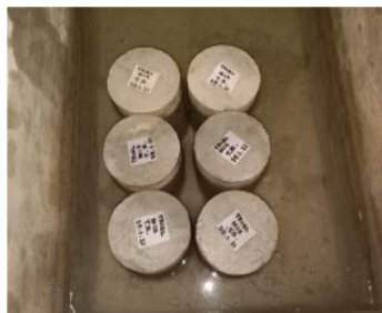
Gambar 4.7 Perendaman Benda Uji Trial Mix
