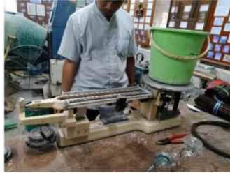
Gambar 4.12 Takar/timbangan Material Campuran Beton
