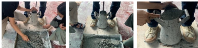
Gambar 4.10 Pengujian Workability Beton ( Slump Test )
