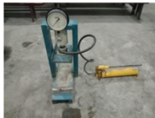
Gambar 3.6 Hydraulic Concrete Beam
