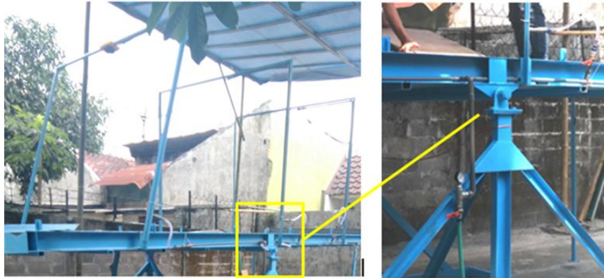
Figure 6. Installation of rainfall simulator on the sloping plot
