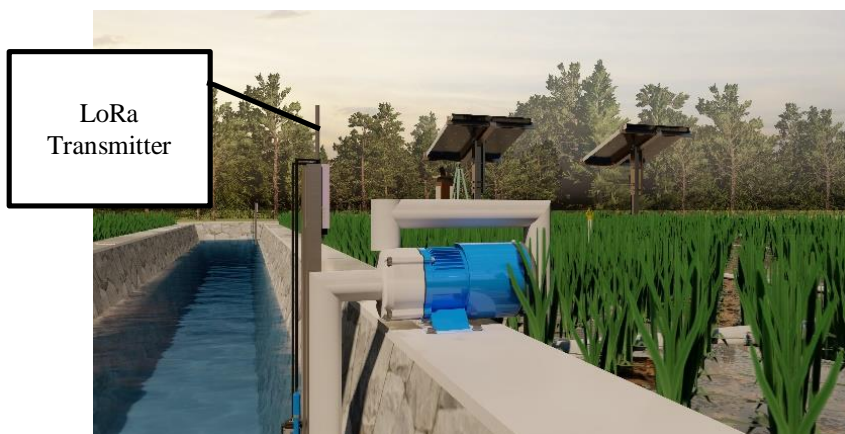
Fig. 4. Water pump used to deliver water to agricultural land
