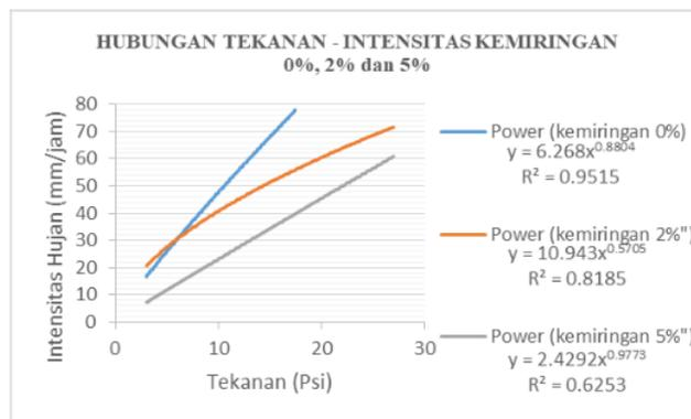
Gambar 2. Kalibrasi Tekanan – Intensitas Kemiringan 0%, 2% Dan 5%
