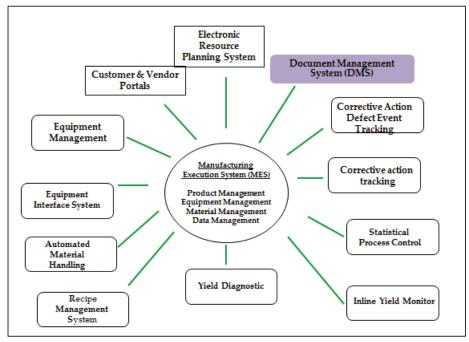
Figure 1: Interlinked manufacturing execution system
