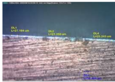
Figure 6. The oxide coating thickness resulted from the anodizing process with a 100% solution type 1M Sulfuric acid ( H_3PO_4 ) with a voltage variation of 30 Volt and immersion time of 10 minutes using an optical microscope 100x
