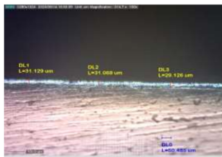
Figure 1. The oxide coating thickness resulted from the anodizing process with a 100% solution type 1M Sulfuric acid (H 2 SO 4 ) with a voltage variation of 15 Volt and immersion time for 10 minutes using a 100x magnification of optical microscopy
