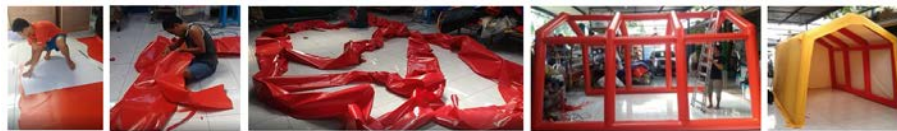
Figure 5: Making an Inflatable Stage Roof (2 weeks)
