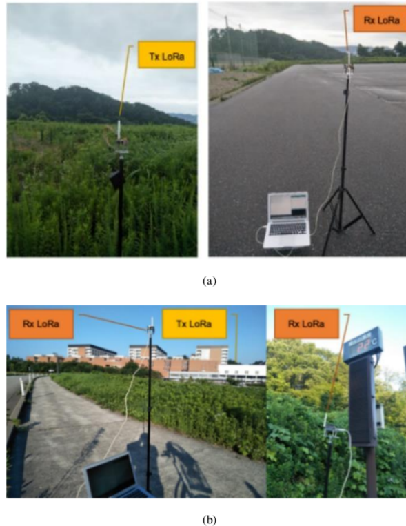
Figure 5. (a) Communication Tx and Rx LoRa 915 MHz on FSPL, (b) Communication Tx and Rx LoRa 915 MHz on Obstacles
