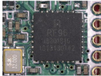
Figure 4. RF96 chip for LoRa 915 MHz from MeRL keyence VHX digital microscope
