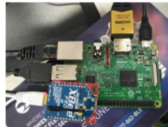
Fig. 12. Raspberry Pi 3 and Zigbee RF Module Connectivity.
